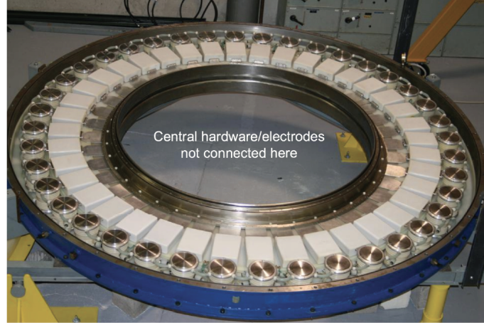
Figure 14: The MAIZE LTD module without any of the stuff in the center. Basically just a big empty electrical donut. Stolen with humility from [4].
